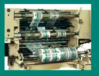
**Slitter** – This is a process where materials are cut or bent with a large machine to specific lengths.
